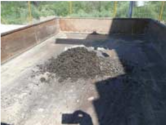
Figure 4.12 Dewatered sludge on trailer
