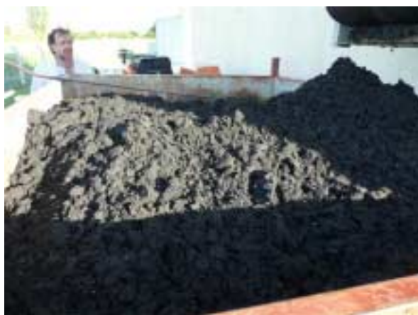
Figure 3.18 Dewatered sludge on trailer
