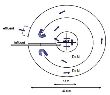
Based on the volumes and a depth of 5 m the total surface needed for the anaerobic tank + activated sludge tank is  $433 \text{ m}^2$ . This results in a diameter of 23.5 m. The diameter of the anaerobic tank should be 7.4 m. The remaining surface is for the activated sludge tank.
