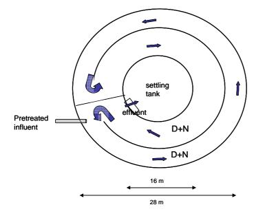
• Example 3: Integrating settling tank with activated sludge tank in a circular reactor
